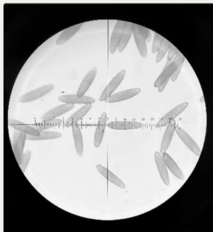
Black soldier fly eggs measured under a calibrated binocular
